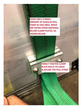
Open the door, install the two washers/nylock nuts on the clamp plate bolts (on the inside of the door). If installing on an insulated door, be cautious to not overtighten the nuts, as this can crush the door panel.
