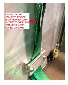
Keeping the strap overlap in place as described, insert the clamp plate bolts through the outer clamp plate and thread them into the inner clamp plate. Barely snug (do not tighten) the bolts.
